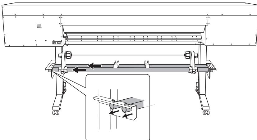
**10** Attach the shaft clamps to secure the shafts in place.**Point**
