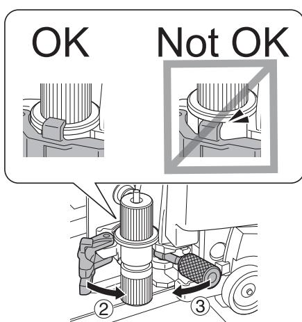
**3** Tighten the screw.
