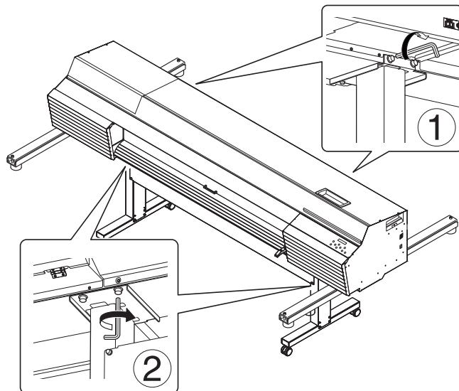
**4 Remove the lifting bars.**
