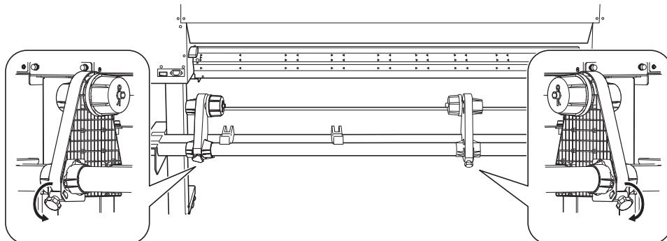
**9** Slide the shafts in to the left side as seen from the rear of the machine.
