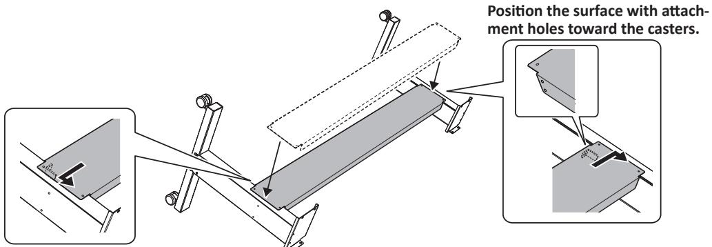
Position the surface with attachment holes toward the casters.
