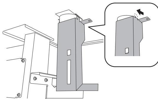
**4 Secure the drain bottle stand in place.**
