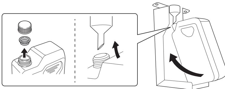
**IMPORTANT: Leave the drain bottle attached at all times.**
