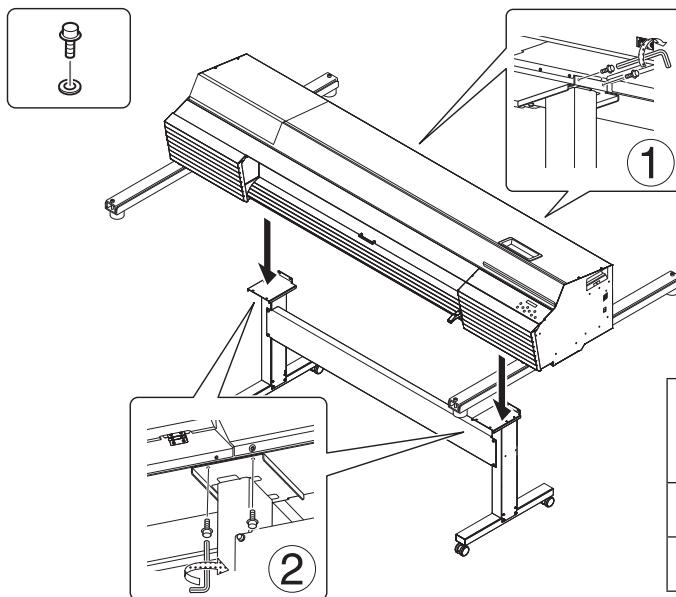
**3 Fully tighten the bolts (long) in the order of ①, ②.**
